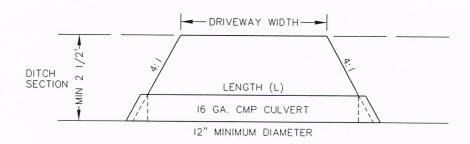
NOTE: THE LIP OF THE CULVERT APRON SHALL BE PLACED AT THE DITCH BOTTOM. IF THE DITCH IS DEEPER THAN THE MINIMUM, THE LENGTH OF THE CULVERT SHALL BE EXTENDED TO MATCH A 4:1 SLOPE.
